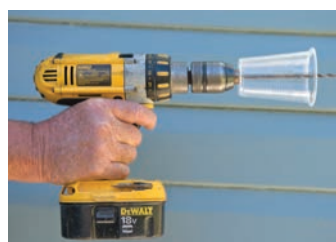
Disposable cup with hole through bottom
