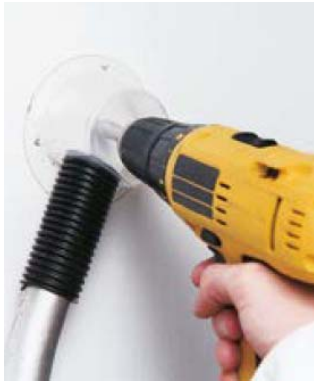
Photo: A vacuum attachment used for drilling in conjunction with a H-Class vacuum cleaner (Source: Health and Safety Executive)
