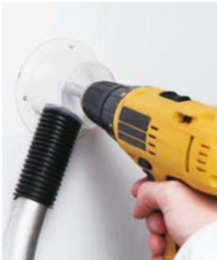
Photo: A vacuum attachment used for drilling in conjunction with H-Class vacuum cleaner. (Source: Health and Safety Executive)
